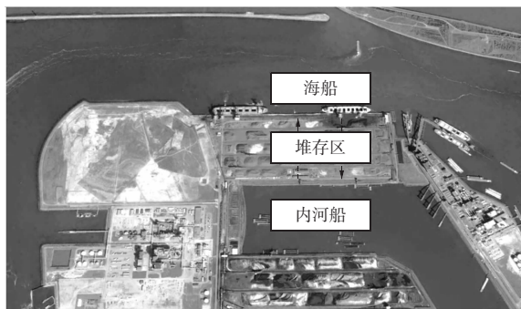
图5 鹿特丹港欧罗波特港区江海联运后方布置形式 Fig. 5 Backside berth layout mode for the river-ocean combined transportation in Europoort area in Rotterdam Port
